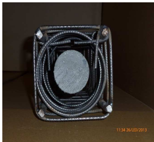
Fig.3: Cross section of complete composite column reinforcement
