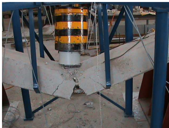
Fig.3: Experiment - crack of specimen under impact
