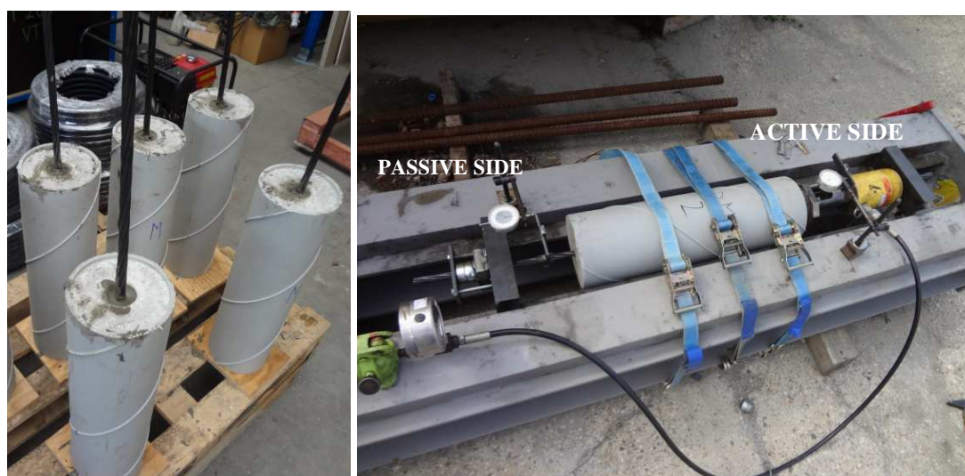
Fig. 3 Hardening of specimens and test arrangement
