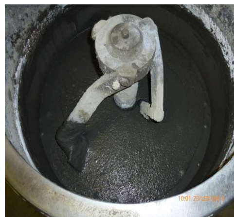
Fig.1: Mixing of UHPC
