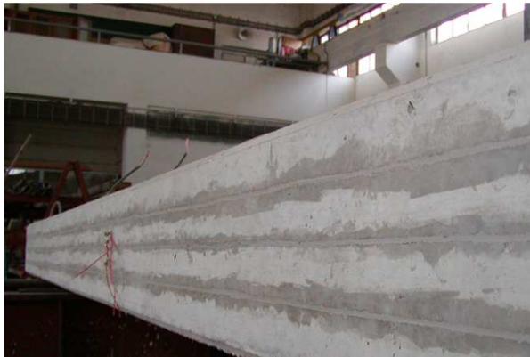
a) NSM CFRP strips
