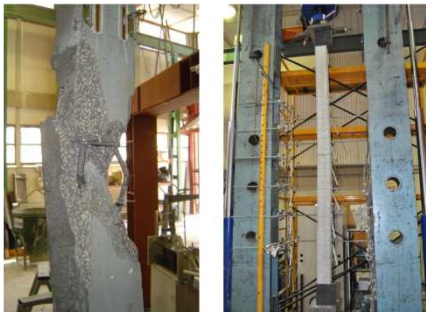
Fig.2: Case of slender column failure
