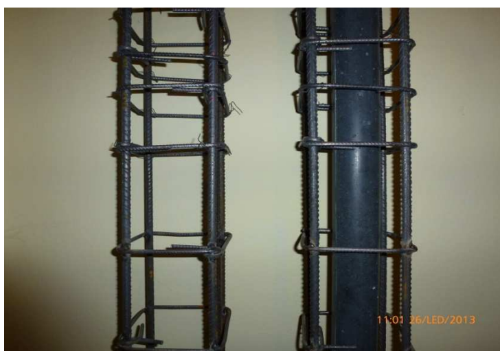
Fig.4: Side view on traditional and composite column reinforcement
